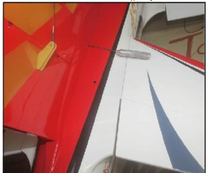
47. Assemble the vertical fin to the fuselage, lock it with screw from the hole in the tail fuselage as picture.
